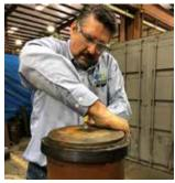
7. Replace clamp and tighten fasteners to secure cellular tube.
