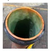
5. Install the new cellular tube. Be sure not to drop in unit as this can damage seals (O-rings).
